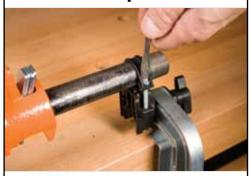
Remove one of the screws from the harness clips on each of the Maxi Clamps. Rotate clip out of the way, and set pipe clamp onto the harnesses. Rotate the clips back over the top of the pipe and secure as shown in photo above.
