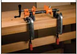
Secure the outer position knobs on both clamps and you are ready to use your pipe clamps clamp for sanding, planing, carving and more.
