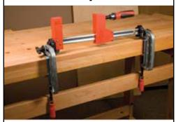
Secure the outer position knobs on both Maxi clamps and you are now ready to use your K-Body parallel clamp for sanding, planing, carving and more.
